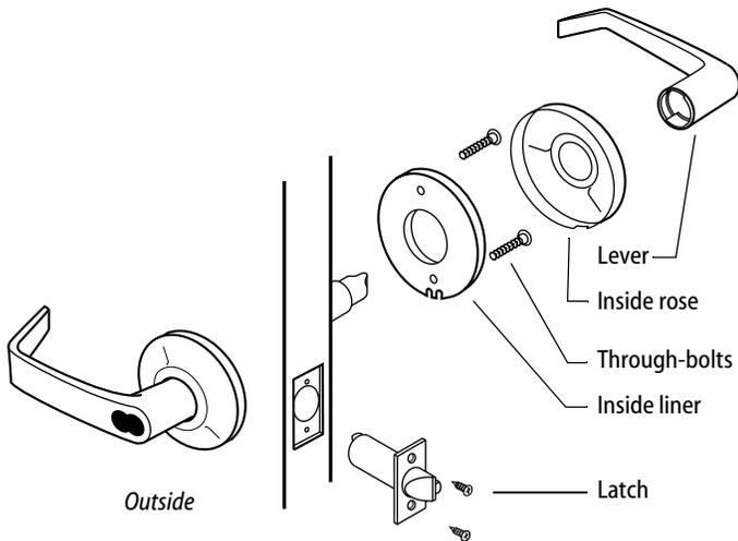
Figure 1 — Overview of installing the lock
