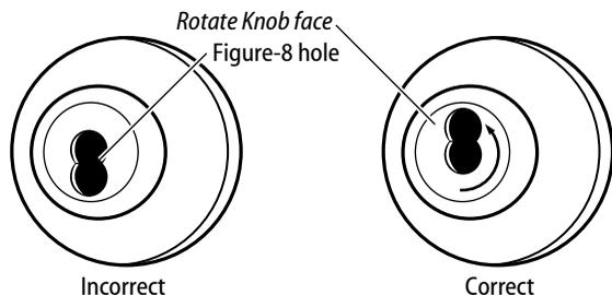
Figure 10 Turning the knob face to correct the handing of the lock
