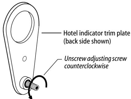
Figure 1 — Unscrewing the hotel indicator adjusting screw
